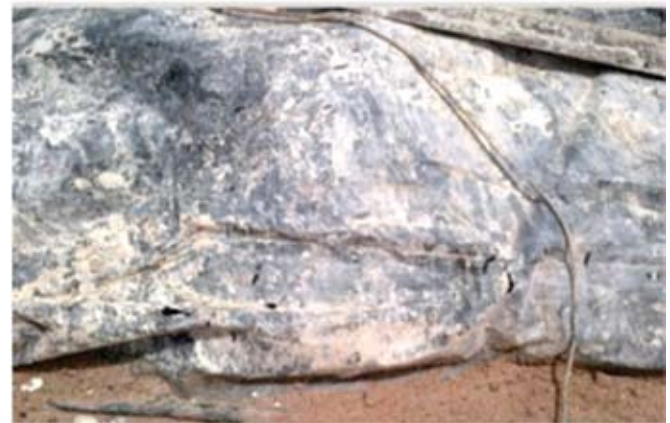
Fig. 3: Photographic view of punctured 250 micron HDPE Liner (Photograph supplied by Areva Renewable Energies India Pvt. Ltd.)
